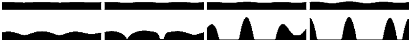
Fig. 2. Snapshots at times t = 10, 12, 13, 14, 15, 15.5, 15.75, 16 for the deterministic thin-film equation. Discretisation parameters are the grid spacing a = 2^{-9} L and time step \tau = a^{5/2} .
