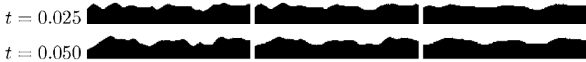
Fig. 4. Film roughness in terms of correlation length l_c : Local snapshots of the film surface at times t = 0.025 and 0.05 for noise strength T = 4.05 \times 10^{-3} and l_c = 0, 0.5, 1 (from left to right). Discretization with a = 2^{-9}L, \tau = a^2 . For the three simulations the same sequence of random numbers have been used.
